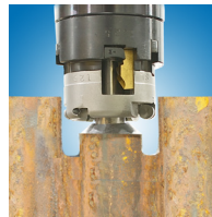
Boiler tube membrane removal and bevel.
